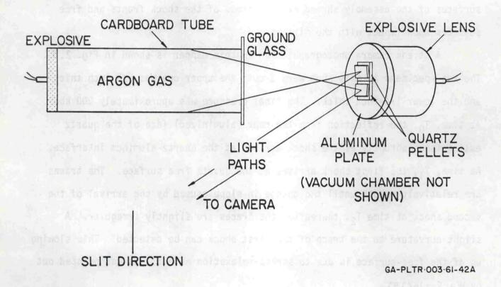
Fig. 2.3.--Diagram Showing Relation of Experimental Assembly, Light Source and Camera.
